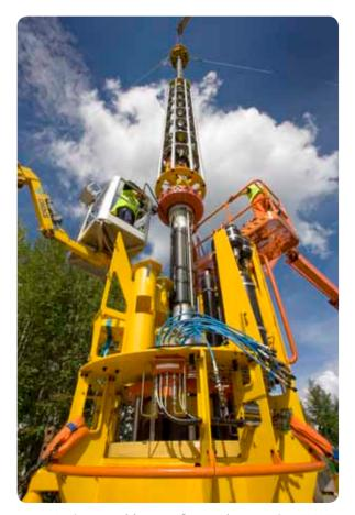
Main assembly test of second generation RLWI
