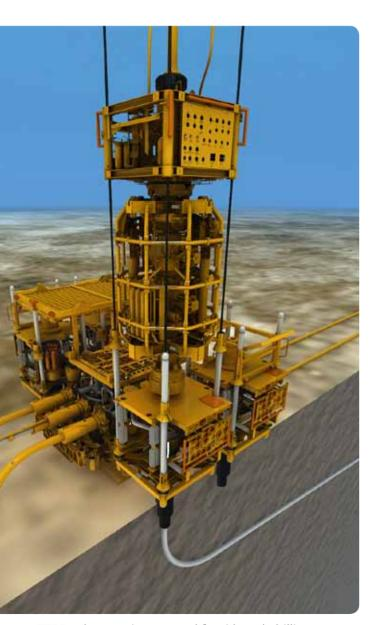
TTRD subsea equipment used for sidetrack drilling
