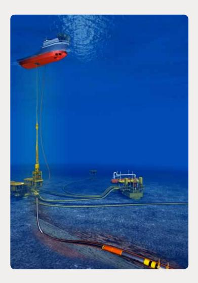
Riserless Light Well Intervention (RLWI) operations are normally carried out from a dynamically-positioned intervention vessel to perform various wireline deployed operations.
