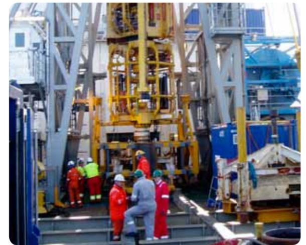
RLWI stack onboard Island Constructor
