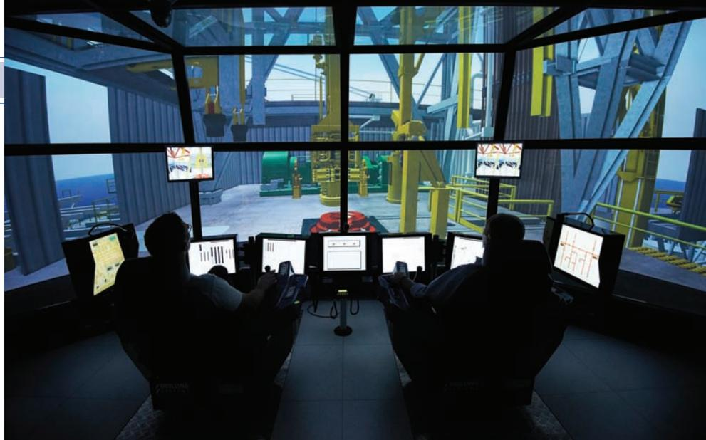
The drilling simulator at Maersk Training, in Svendborg, Denmark, will be used to train crews working on 20K-capable drilling rigs. (Image courtesy Maersk)
