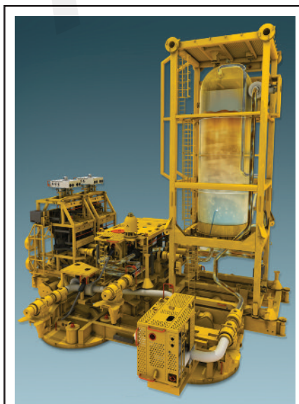
The subsea processing system on Total's landmark deepwater Pazflor project offshore Angola includes seafloor gas/liquid separation utilizing vertical vessels to separate gas from liquid in the production stream. Each separator vessel is about nine meters tall and 3.5 meters in diameter.
