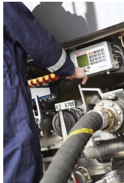
A driver in Europe keys data into the computerized cargo security system on a petroleum tank truck. Used for years in Europe, these systems are getting fresh attention in the United States as gasoline and diesel prices climbed steadily over the past couple of years. Cargo theft is becoming a growing concern for fuel haulers.
