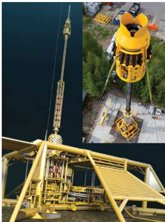
Mark II riserless light well intervention system.
