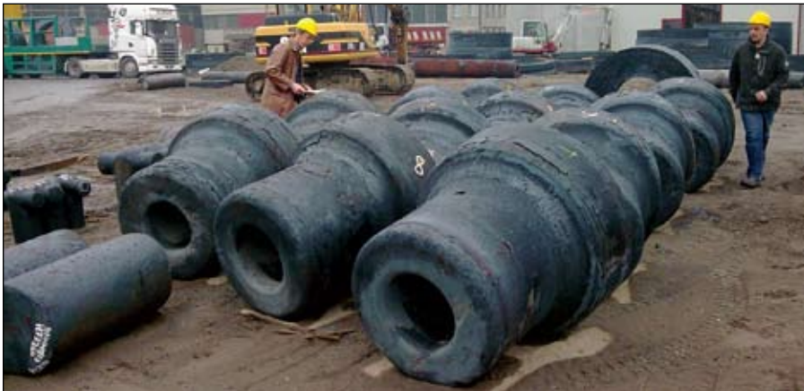
Venture Production helped to develop a new high-pressure riser that uses shrink-fit technology to connect the pipe and flange to avoid welding problems.
