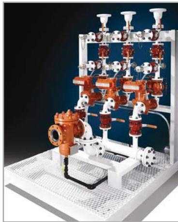
Atie-in skid is a configuration of equipment that is used at an existing loading rack to “tie-in” ethanol or B100 to be either blended or loaded as straight product into a transport. This skid has a four-inch feed line that is split into three, two-inch supply lines for the loading rack.
